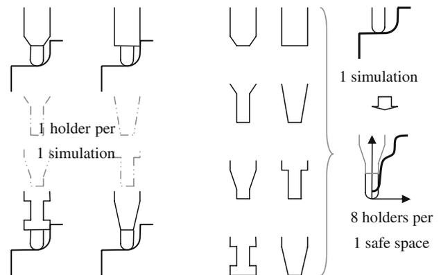
a Collision check by simulation      b Collision check by safe space
