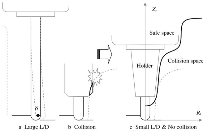
Fig. 1 Short and safe tool setting by safe space
