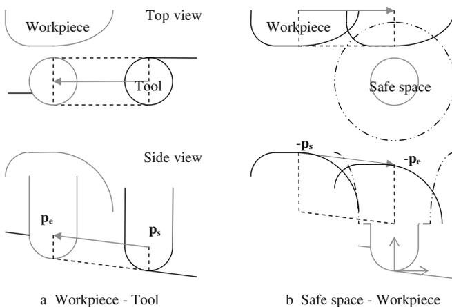
**Fig. 2** Boolean operation between workpiece, tool, and safe space
