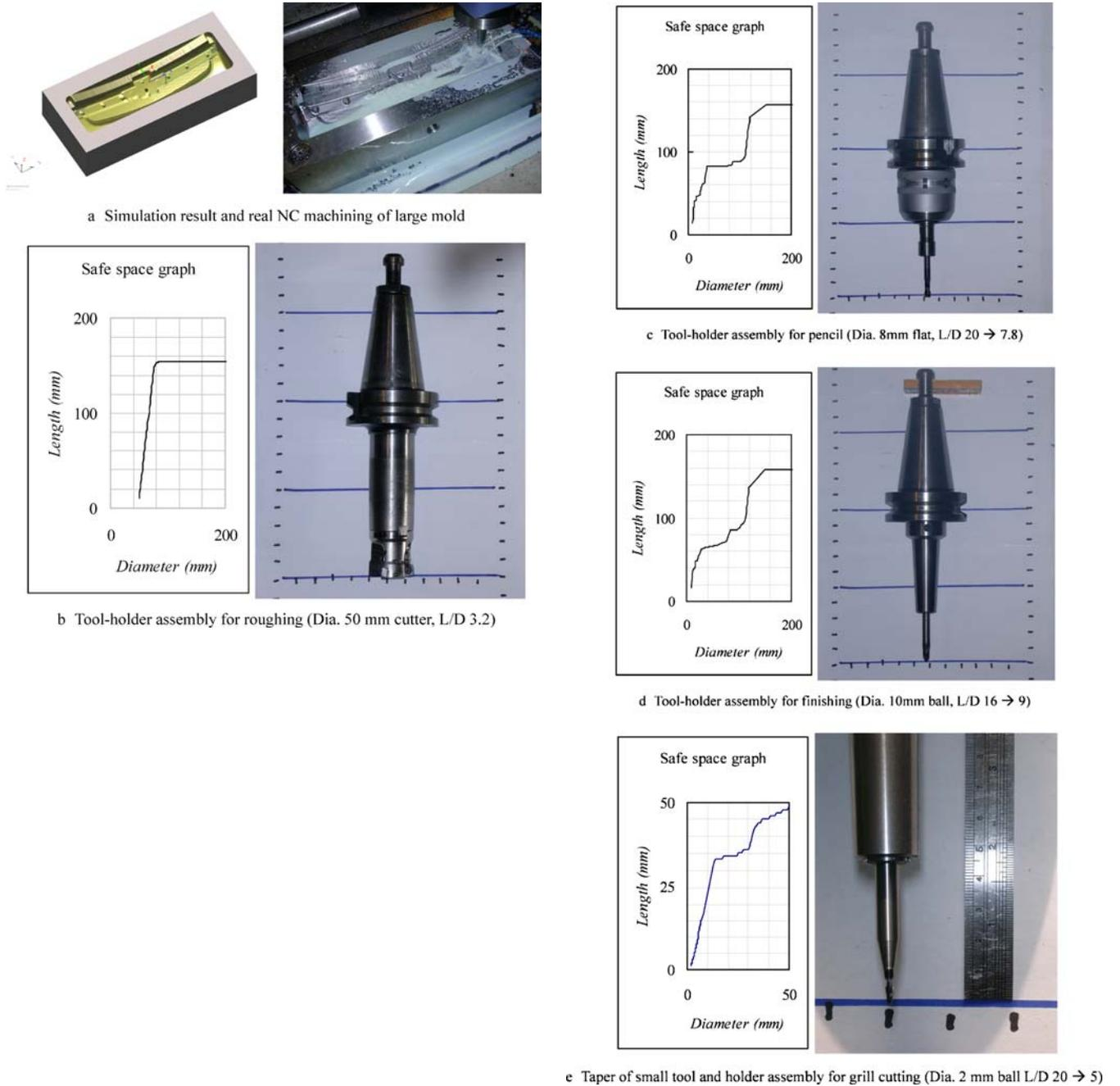
**Fig. 6** Experiment of tool-holder setting method using safe space; on the *left* is the safe space graph and on the *right* is the tool holder and arbor assembly used in NC machining
