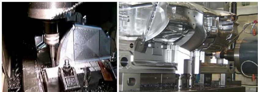
a The slide core of mold
