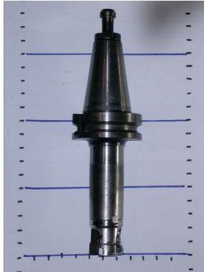
(b) Tool-holder assembly for roughing (Dia. 50 mm cutter, L/D 3.2)
