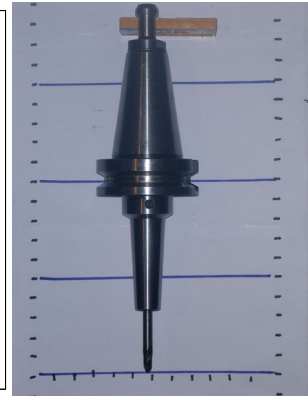
(d) Tool-holder assembly for finishing (Dia. 10mm ball, L/D 16 → 9)
