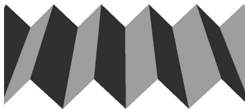
(b) Finishing step, 2d \cdot \tan\left(\frac{a}{2}\right) \geq p
