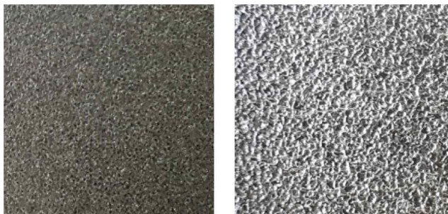
(a) I=1 A Ra=1.13 \mu m (b) I=5 A Ra=3.08 \mu m
