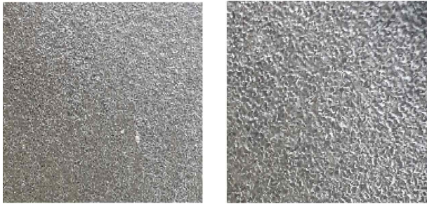
(a) Company Ra = 1.99 μm (b) Suggested Ra = 2.29
