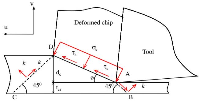
Fig. 2 Determination of the critical thickness  $t_{cr}$
