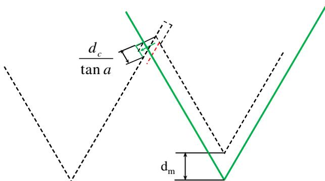
**Fig. 4** Side burr formation at final depth
