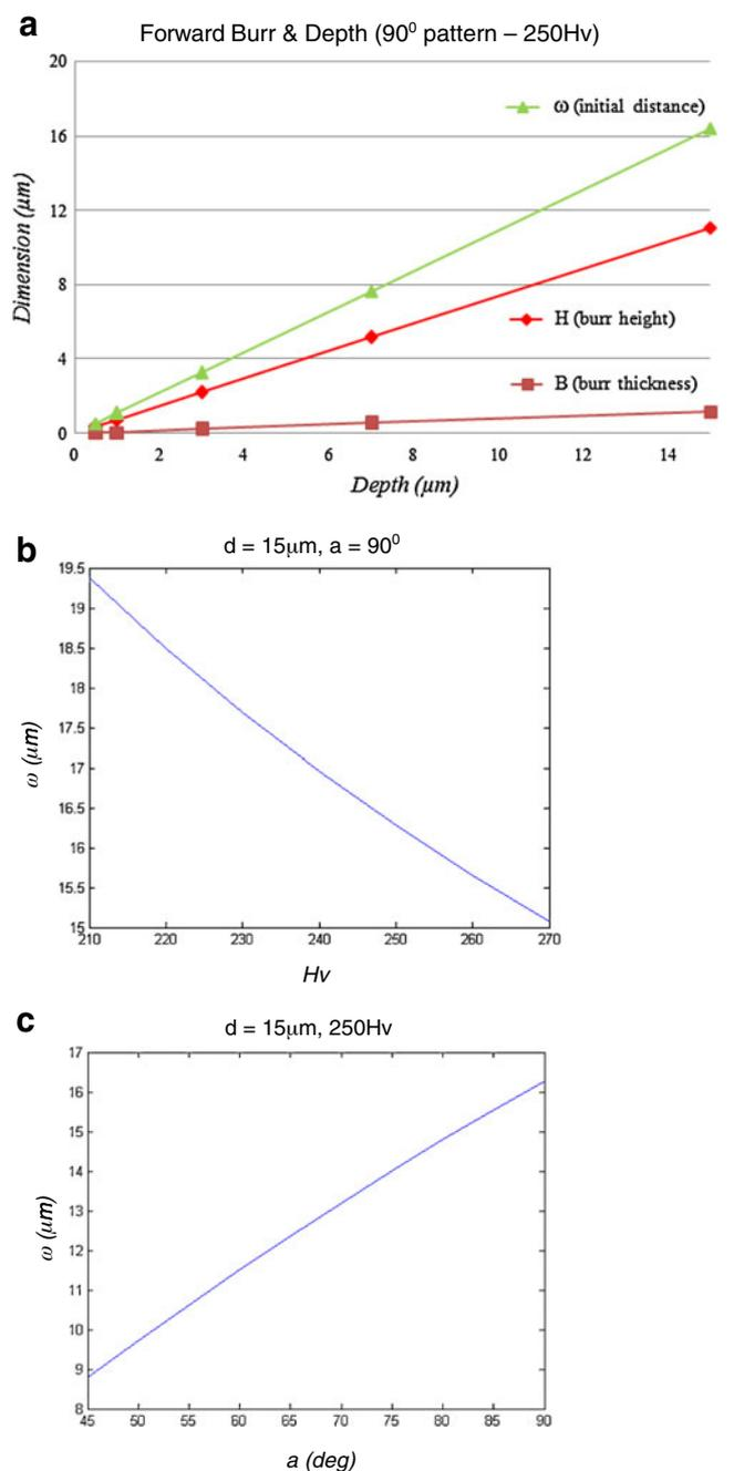
**Fig. 12** Predicted results on exit burr of pyramid pattern. **a** Exit burr and cutting depth,  $V$  90°, 250 Hv. **b** Initial distance and Hv. **c** Initial distance and pattern angle
