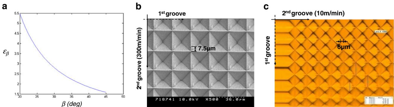
**Fig. 14** Comparison between prediction and experiment on exit break off in pyramid pattern. **a** Prediction of  $\beta$  till break off occur with  $\epsilon_f=1.2$ . **b** Break off size with  $v_c=300$  m/min. **c** Break off size with  $v_c=10$  m/min
