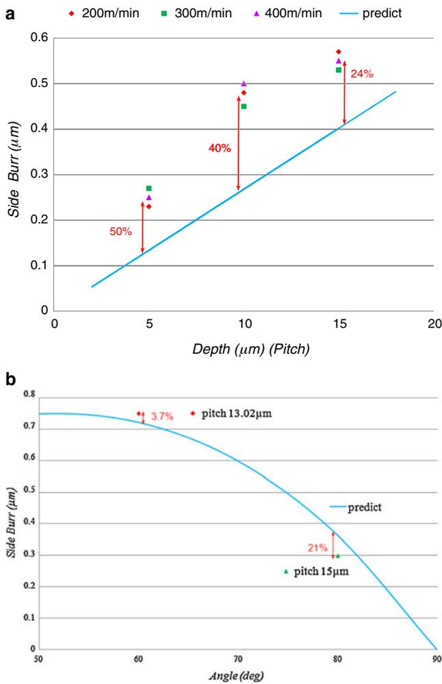
**Fig. 11** Comparison between prediction and experiment on side burr of prism pattern. **a** Single grooving, depth = pitch,  $V$  80°, 210 Hv. **b** Two-step grooving, 300 m/min, 210 Hv
