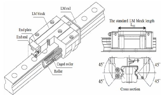
Fig. 1. Schematic of the roller linear motion guide [20].
