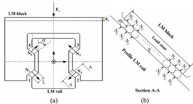
Fig. 2. Contact force of the roller linear motion guide and Sec. AA along the perpendicular direction.
